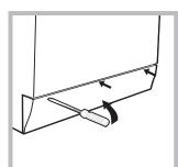
1. using a screwdriver, remove the cover panel on the lower front part of the washer-dryer (see figure);
